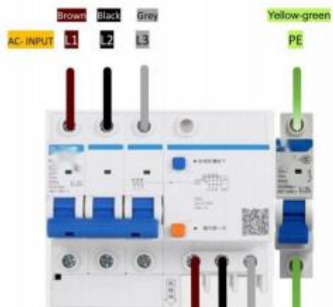
Schematic diagram of L1, L2, L3, PE input wiring
