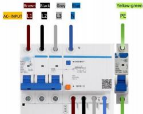
Schematic diagram of L1, L2, L3, N, and PE input wiring
